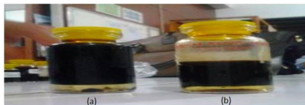
Figure 2. The organic liquid product (OLP) of Nyamplung oil cracking using a combined catalyst of Zn-HZSM5 and \gamma Alumina with composition (1: 3) at (a) Temperature 300 °C ; (b) Temperature 350 °C
