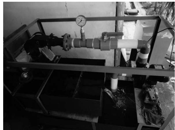
Figure-3. Penguajian turbine drive Generator.
